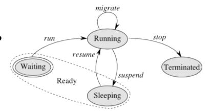
A cluster-wide context switch (a set of VM context switches) enables to efficiently rebalance the cluster according to the: scheduler objectives / available resources / waiting vjobs queue (elasticity) [VTDC 2010]
